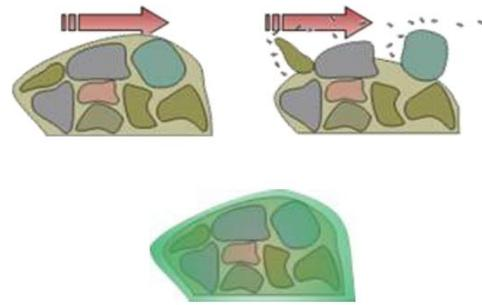
Fig. 5: Principle of sand consolidation by microgel/polymer treatment
