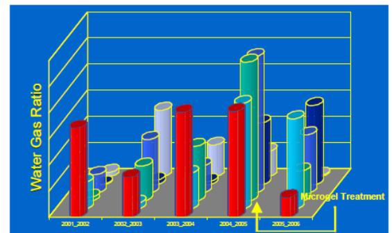
Fig. 6: Evolution of water-to-gas ratio after microgel treatment of gas storage well (Zaitoun et al., SPE 106042, 2007)
