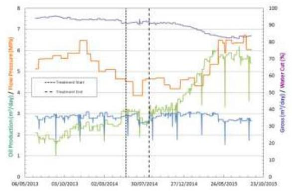
Fig. 7: Microgel Conformance treatment. Response on offset producing well (Dupuis et al., SPE 179765, 2016)
