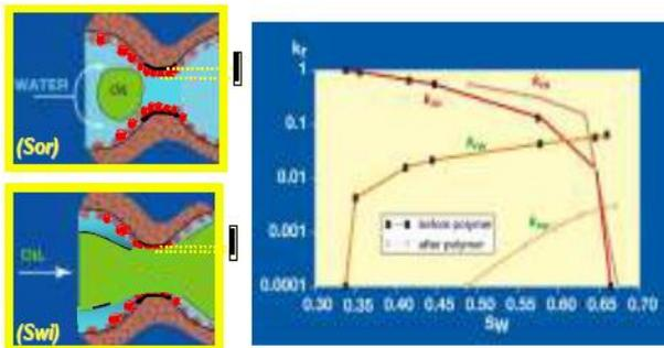
Fig. 2: RPM mechanism induced by microgel/polymer adsorption.
