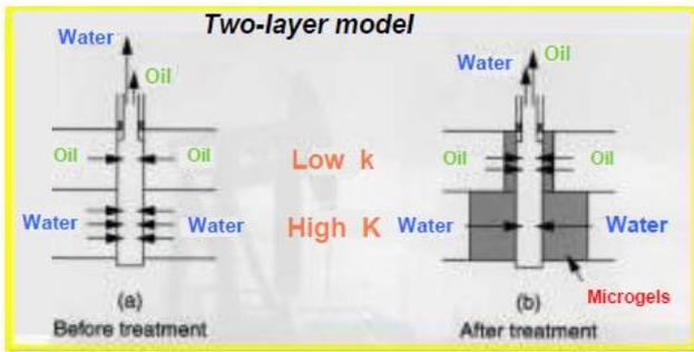
Fig. 1: Principle of production well water shut-off treatment by polymer (Zaitoun et al., SPE 56740, 1999)
