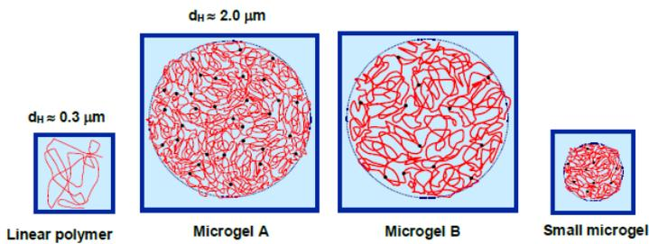
Fig. 3: Comparison of microgel species with high-molecular-weight linear polymer.
