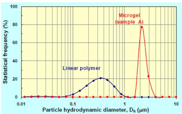
Fig. 4: Size distribution of microgel and polymer measured by Dynamic Light Scattering (PCS).
